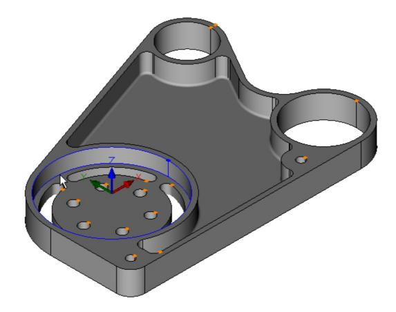
Press the escape key to deselect the bore Contour. Highlight and select the slots and holes in the bore: One of the slots is obscured, choose the Top View command to assist in selection. Menu: View -> Top View Toolbar button:
