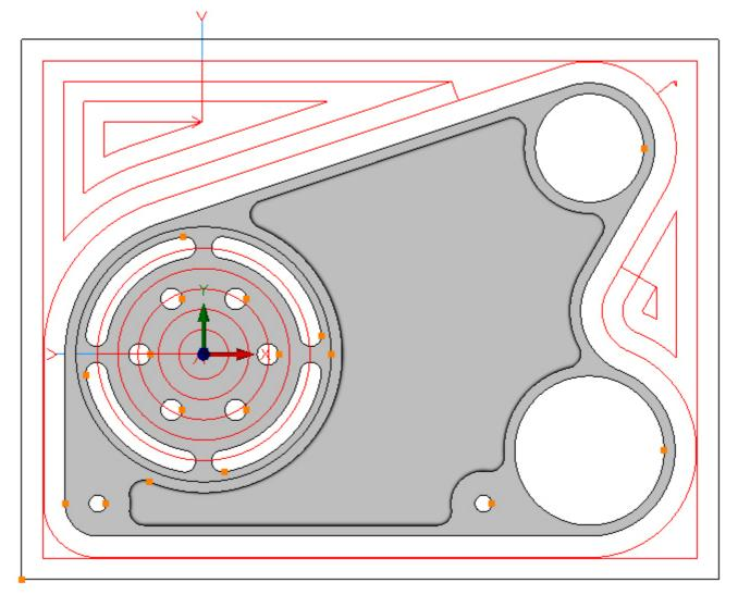
This time Smart Ramp is required, this is still unchecked from the previous pocketing operation. Choose the Entry tab and check Smart Ramp:
