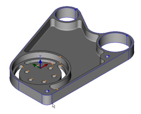
• Press the escape key to deselect the Contours and exit the Set Contour Height command. Highlight and select the inner pocket Contour:
