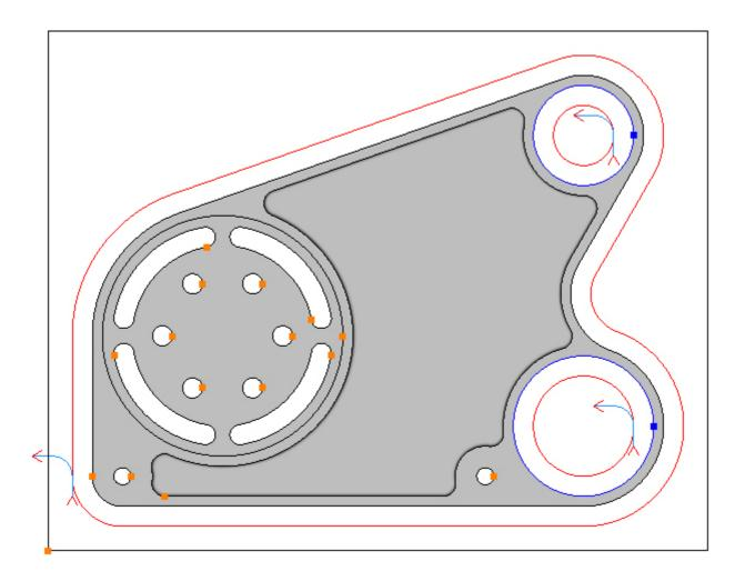
Change the entry and exit because the settings from the previous operation are still in effect. Choose the Entry tab and set the values (before checking the boxes) as below and check the line and arc check box:
