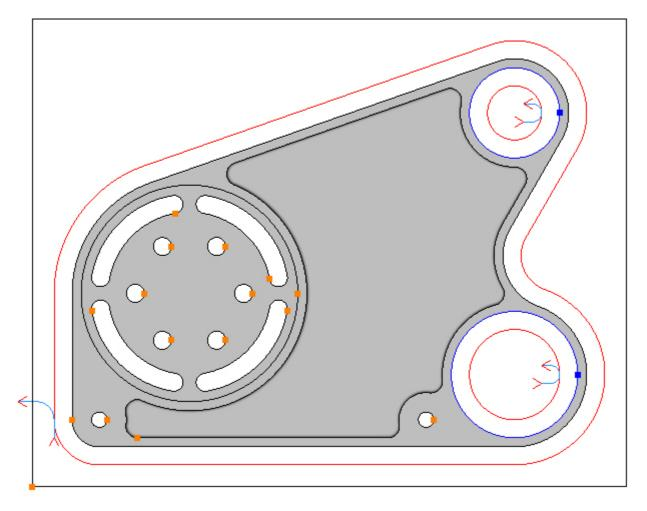
Cutter radius compensation is required for this profile operation. Choose the Cutting Data tab and select *Control Tool Centre*, if not already selected:
