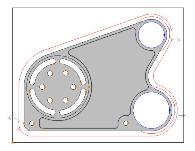
As can be seen the toolpaths are on the outside and in a clockwise direction, this is the default. This needs to be changed to the inside in a counter-clockwise direction. The Contours must be selected in order to change the side and direction of the resulting toolpaths. When Contours are added to an operation they will be left selected. If the Contours are not selected they must be selected first, they can also be selected by clicking the name in *Contours* group box:
