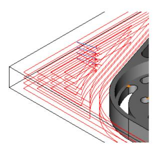
Choose the Entry tab and uncheck the Smart Ramp check box and check the Line check box:
