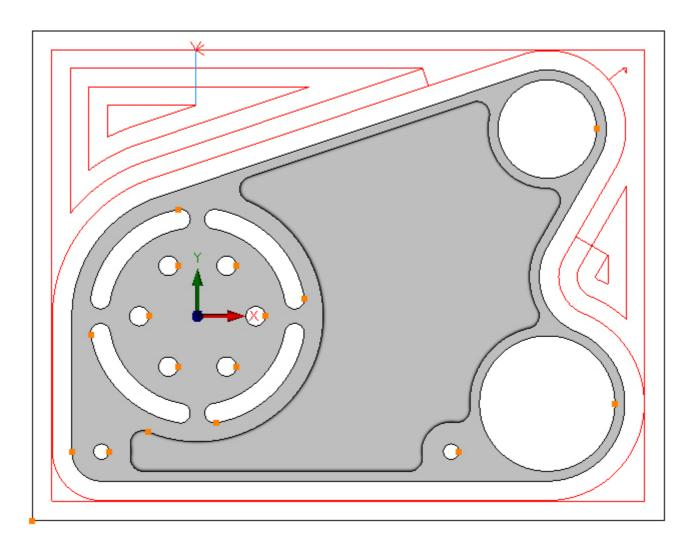
Looking at the resulting toolpaths a blue line can be seen in the top left hand corner. Blue indicates an Entry, the entry is configured using the Entry tab:
