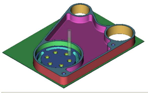
Simulating the Part is optional and does not need to be performed to create the Nc code.
