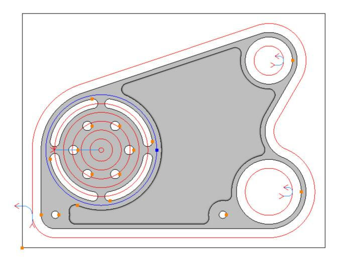
Smart Ramp is applied, but is not particularly suitable as the cutter will plunge against the side wall. Choose the Entry tab, uncheck the Smart Ramp and change the line length to 1. Check the Line (if not already selected) and then the Ramp check box:
