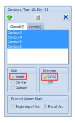
The toolpath is now on the inside and in counter-clockwise direction:
