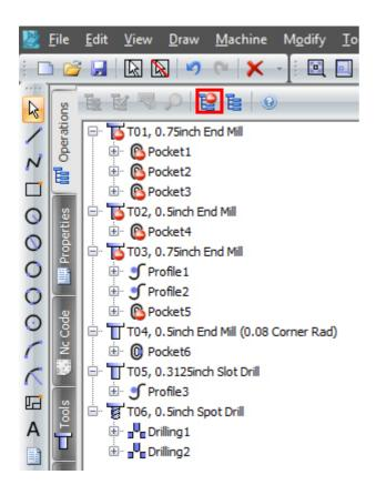
Click the Properties tab on the Part Manager to continue with the Drilling command:
