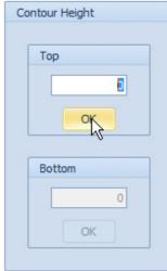
Pick the Bottom value from the model. Highlight a point on the bottom edge of the bore:
