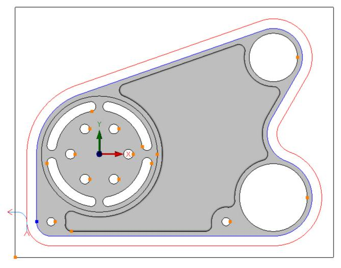
Cutter radius compensation is required for this profile operation. Choose the Cutting Data tab and select *Control Tool Centre*:
