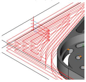
To start further outside of the billet increase the length of the entry line. Change the entry line length, for example, to 2 (2 x the tool radius = 0.75):
