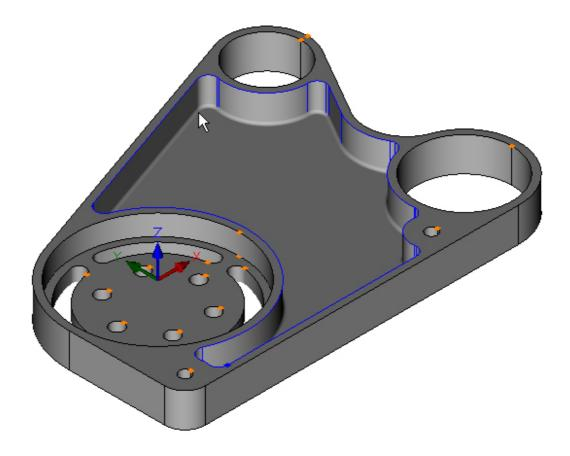
The bottom of the Contour is hidden by the radius in the corner, you can set the view to Wire Frame to see the bottom of the Contour: Menu: View -> Wire Frame View Toolbar button:
