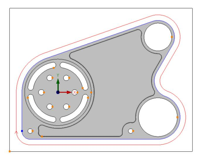
Add an entry and exit. Choose the Entry tab and change the Line/Arc Angle to 0 and check the Line check box:
