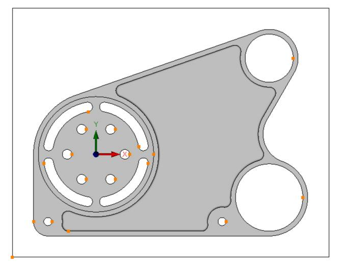
By default the Contour that forms the rectangle has a Z Top and Z bottom of zero. The outside profile and the rectangle will be used for the pocketing operation, they both must have the same Z Top and Z bottom.
