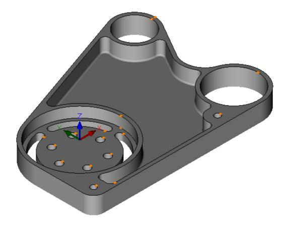
• Highlight outer Contour on top face, left click to select, repeat for four circles on top face also:
