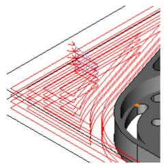
As can be seen the Smart Ramp, as the name implies, automatically ramps to depth at the shallowest angle possible. As it is the outside profile that is being machined Smart Ramp is not needed, because it is possible to plunge to depth outside of the billet. First start from the outside, click the Advanced tab:
