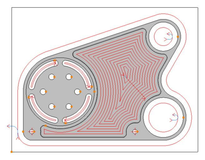
As the Z position of the  $\emptyset 0.375$  holes are different a new drilling operation is required. Menu: Machine-> Drilling
