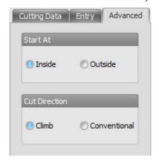
At the moment the pocketing starts from the inside, click the outside radio button and the toolpaths will be recalculated to start from the outside:
