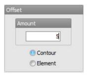
Move the cursor over the Ø120 circle and left mouse click to indicate that the offset is to be from this circle, then left click on the outside of the circle to create the offset; repeat for the Ø50 and Ø70 circles:
