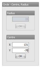
Create a second circle of the same radius but using snap to centre. Move the cursor over the 15mm radius, not near the end or mid point, until the Center snap symbol is showing and a blue Snap Marker indicates the Snap Point. It may be necessary to zoom in on the 15mm radius by pointing the cursor at it and rotating the middle mouse button:
