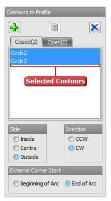
To change the side and direction click the appropriate radio button, in this case *Inside* and *CCW*:
